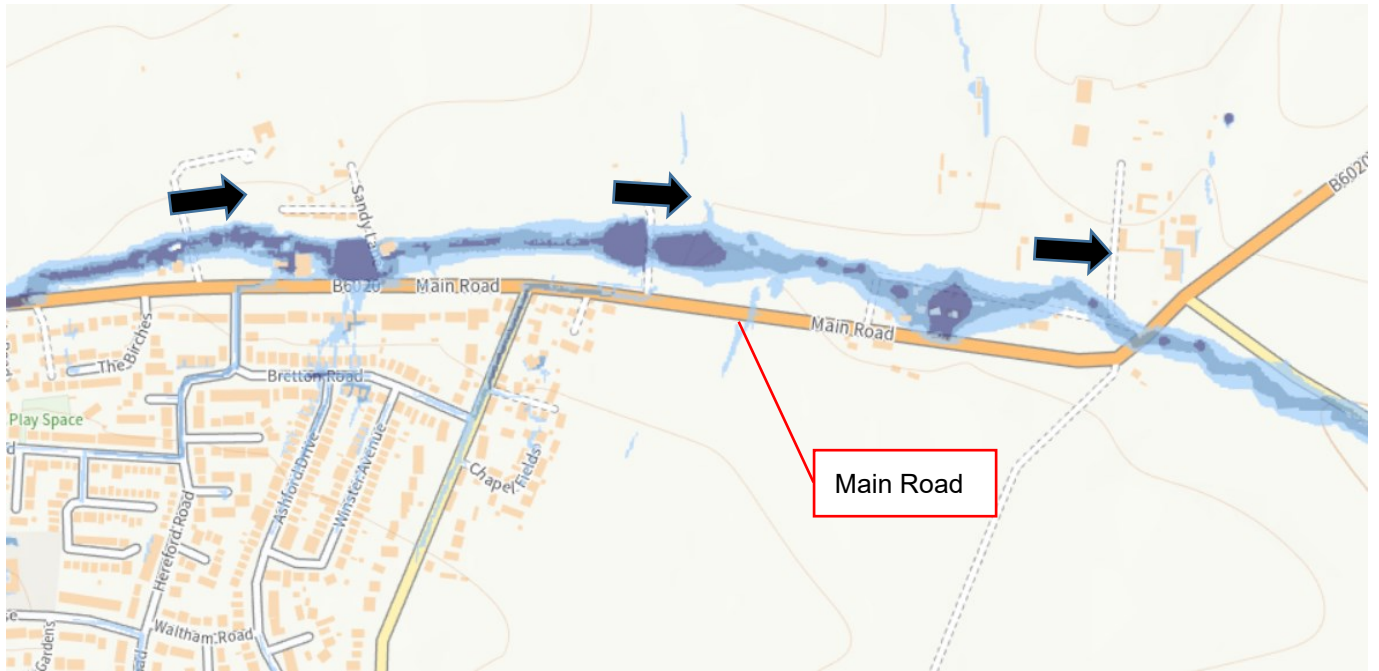
Figure 3. Predicted Surface Water Flood Extents – Main Road
